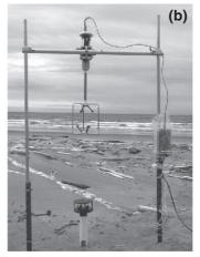
**Fig. 17.9** (a) A typical 10 m meterological mast with sensitive 3-cup anemometers and wind vanes mounted logarithmically (b) three dimensional (*upper*) and two dimensional (*lower*) sonic anemometers mount on an 'H' frame
